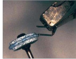
Fig 6. Smoothing the cut legs of the male attachment
